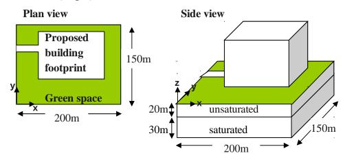
Engineers are estimating the area of green space needed for a new housing development to meet NYC's policy to increase infiltration and reduce runoff.
